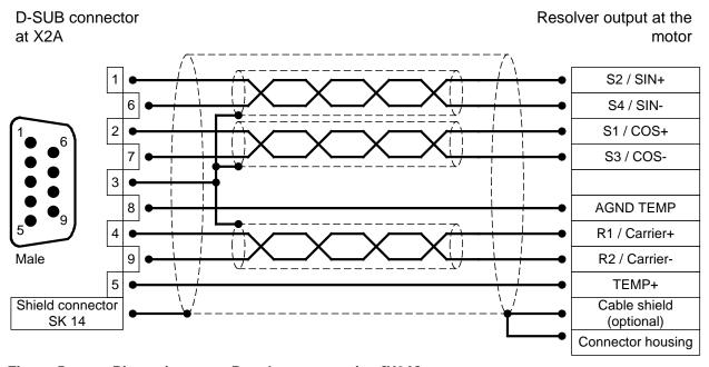
Figure 5: Pin assignment: Resolver connection [X2A]
