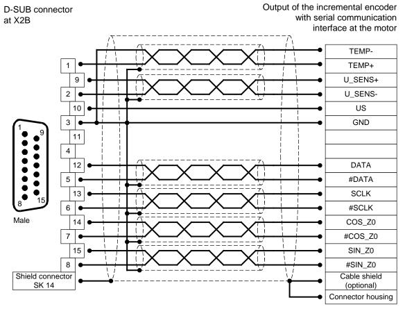
Figure 8: Pin assignment: Incremental encoder with serial communication interface (for example EnDat, HIPERFACE®) [X2B]
