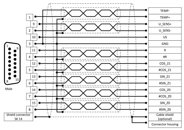
Figure 6: Pin assignment: Analog incremental encoder [X2B]
