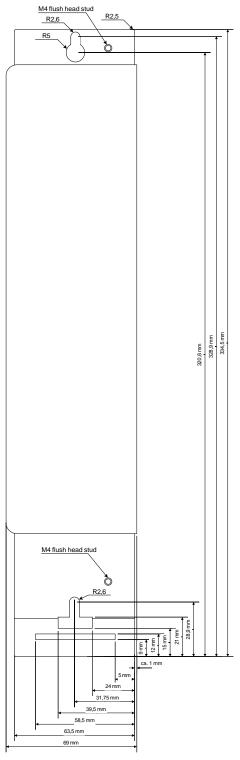
Figure 4: Servo drive ARS 2300 SE: Mounting plate
