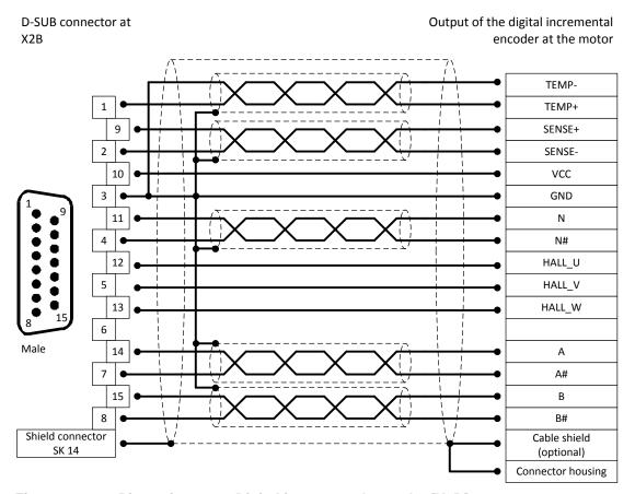
Figure 9: Pin assignment: Digital incremental encoder [X2B]
