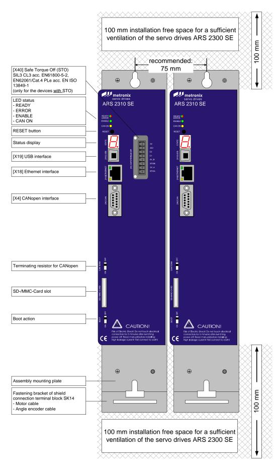
Figure 1: Servo drive ARS 2300 SE with and without STO: Front view – Installation free space and mounting distance
