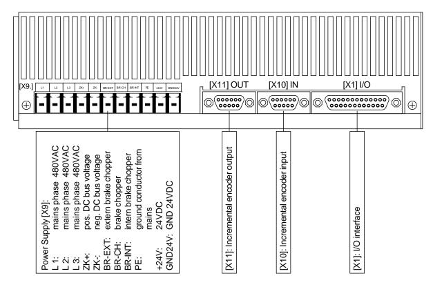
Figure 2: Servo drive ARS 2302 SE: Top view
