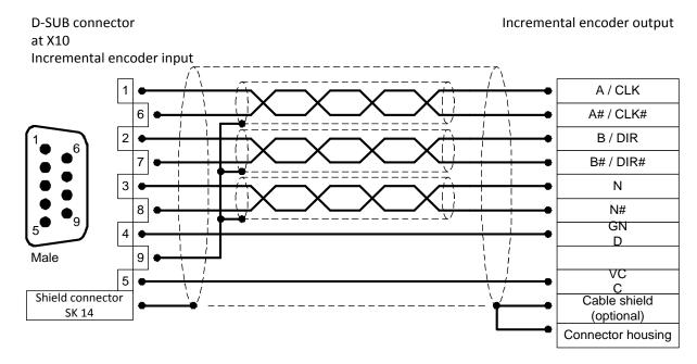
Figure 14: Pin assignment: Incremental Encoder Input [X10]
