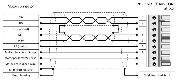
Figure 13: Motor connection [X6]
